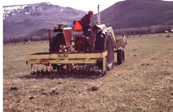
**Fig. 8. An AerWay® aerator is used to punch slots in the existing sod as the teeth, which are approximately 8 inches in length, roll across the ground. (Photo by Joe Brummer)**
