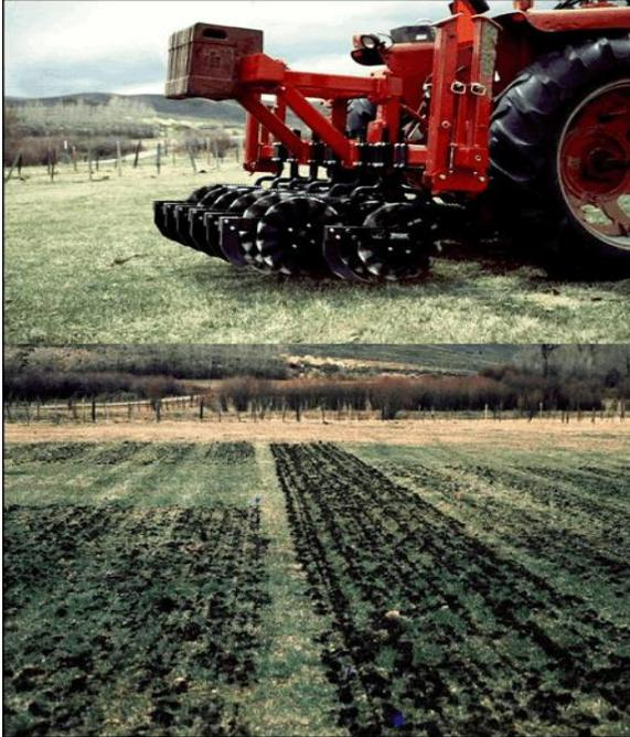
**Fig. 9.** A homemade ripper-type aerator (top photo) being used to cut slots (bottom photo) about 4 inches deep every 6 inches in the existing sod of a mountain meadow. In this trial, ripping reduced hay yields by over 30%. (Photos by Joe Brummer)
